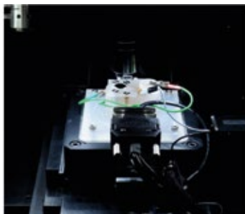
Fig. 1: Novel back-side hydrogen charging setup developed in-house for in situ micromechanics during hydrogen charging and transmission electron microscopy image of a deformed microstructure after nanoindentation under the influence of hydrogen.
