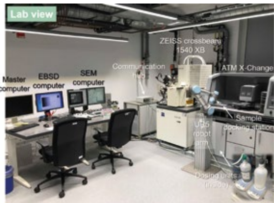
Fig. 1: Overview on the large-volume 3D EBSD setup based on chemo-mechanical serial sectioning.
