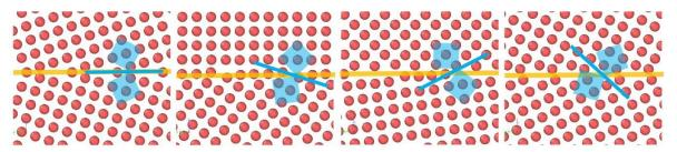
Even the mere tilt in the grain boundary plane with identical misorientation impacts the chemical composition and atomic arrangement of the microstructure and makes the material more or less prone to failure. Visualized here is the angle between the grain boundary plane and the internal bisector between the [0 0 1] directions in the grains. Copyright: X. Zhou, Max-Planck-Institut für Eisenforschung GmbH
