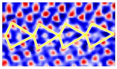
Transmission electron microscopy image resolving even light atoms (here: boron and carbon) as interstitial atoms in the centre of the atomic motif. Image taken from <a href="https://doi.org/10.1038/s41467-023-39302-x">https://doi.org/10.1038/s41467-023-39302-x</a>
