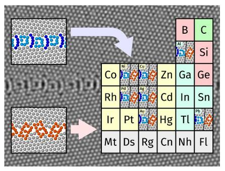
Two different families of grain boundary structures first discovered in copper were investigated in a range of fcc metals via atomistic computer simulations. The "domino" (red) and "pearl" (blue) motifs were found to be universal to the investigated fcc metals. Copyright: T. Brink, L. Langenohl, Max-Planck-Institut für Eisenforschung GmbH
