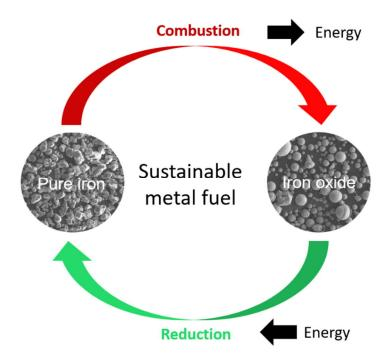
Energy is stored while reducing iron oxide to iron. Energy is freed while combusting iron back to iron oxide. Optimizing this process could lead to a fully circular, thus sustainable storage of energy. Copyright: Laurine Choisez, Max-Planck-Institut für Eisenforschung GmbH
