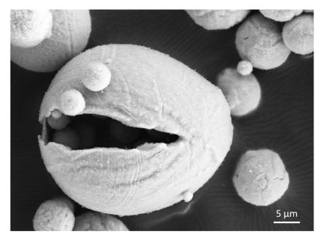
Iron powder combusted in an industrial-scale burner, used for the application of sustainable energy carrier. Copyright: Laurine Choisez, Max-Planck-Institut für Eisenforschung GmbH Original publication:
