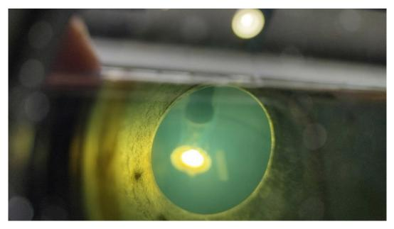
Inside an arc furnace at the MPIE: the bright light in the middle shows the molten iron oxide. The surrounding greenish light shows the hydrogen plasma. The project "ROC" is funded through an Advanced Grant of the European Research Council and aims to produce steel in one single step with hydrogen-plasma instead of carbon. This method would reduce the worldwide carbon emissions by 8%. Copyright: Max-Planck-Institut für Eisenforschung GmbH
