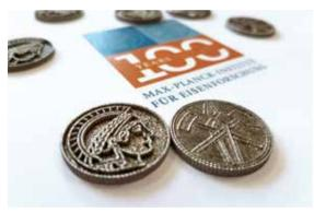
One example of the complexity of components that can be produced by additive manufacturing: the logo of the Max-Planck-Institut für Eisenforschung as a relief on 3D printed coins of stainless steel.
