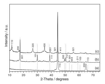
**Figure 3.** GI-XRD patterns of (a) the bare metal (pure iron; JCPDF no. 06-0696) before exposure to the saline  $H_2S$  saturated acetic solution, (b) the electrochemically grown corrosion products (mackinawite; JCPDF no. 15-0037), including lines showing position and relative intensities based on JCPDF no.15-0037 for mackinawite, and (c) the corrosion products after exposure to air for 90 d (akaganeite; JCPDF no. 34-1266).
