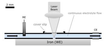
**Figure 1.** Scheme of electrochemical cell used for in situ Raman measurements (cell thickness 1 mm; cover slip thickness 0.2 mm; tubing diameter 0.6 mm; electrode area 0.2 cm<sup>2</sup>).
