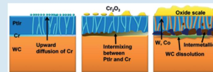
Fig. 4: Schematic illustration of the evolution of degradation.
