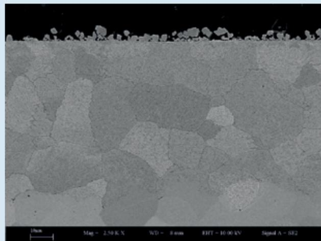
Fig. 1: SEM image of a Fe-2Mn-2%Si model alloy annealed at 700°C for 70 hours at partial pressure of oxygen just below the equilibrium partial pressure of Fe/FeO.
