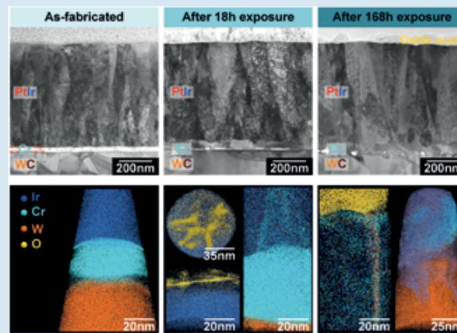
Fig. 3: Cross-sectional STEM images and APT analysis of specimens after different periods of isothermal exposure at 630°C under an oxidizing atmosphere ( $P_{O_2} \approx 1.12 \times 10^{-23}$  bar).
