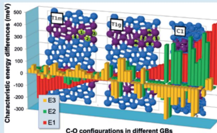
Fig. 2: Comparison of various C-O configurations in five different grain boundaries (GBs) in hcp Ti with (E1, red) O and C solved in the grain interior; (E2, green) O and C independently segregated to grain boundaries; and (E3) the pair formation in the grain interior (E3, yellow). Negative energy differences favour the formation of these configurations.
