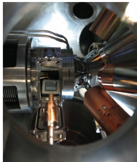
Fig. 2: Photo of the reaction cell inside the UHV chamber: It is docked with the differentially pumped analyzer and opened for sample transfer.
