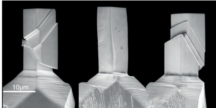
Fig. 1: Example of compressed copper micro pillars. The pillars in (a,c) are single crystalline with clear slip steps through the entire pillar documenting free glide of dislocations. The centered pillar (b) is comprised from the two single crystalline ones at the side, with a grain boundary in the center. Many more faint slip steps document the important role of grain boundaries as obstacles for dislocation motion.
