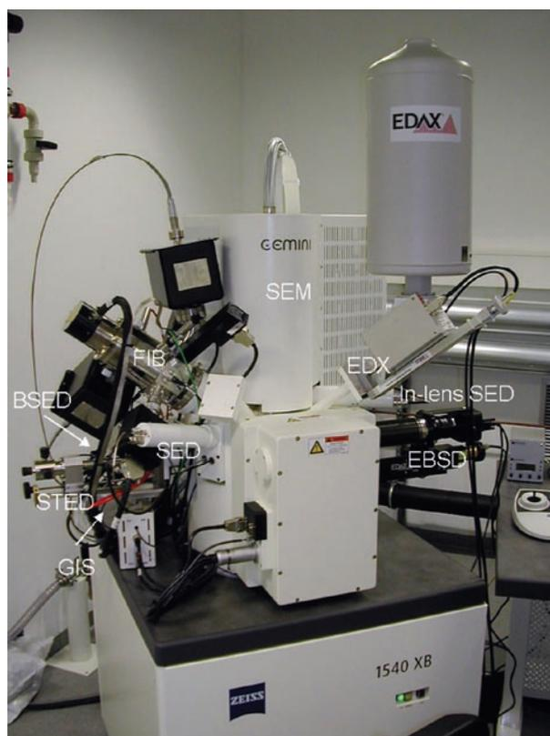
Fig. 4: FIB-SEM column with the various detectors marked.
