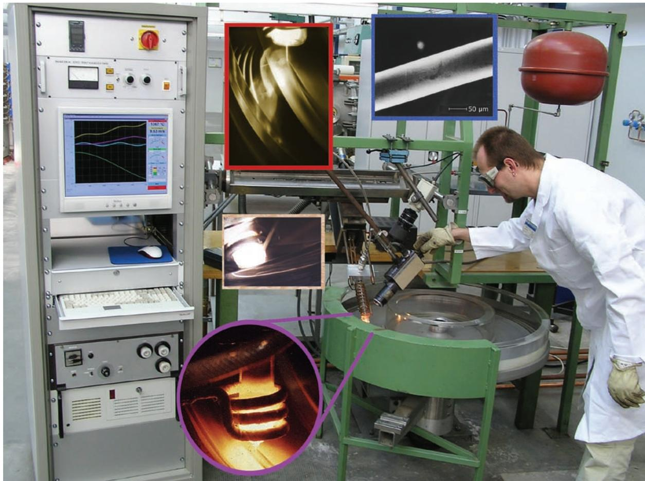
Fig. 15: In-rotating-liquid-spinning (INROLISP) facility.
