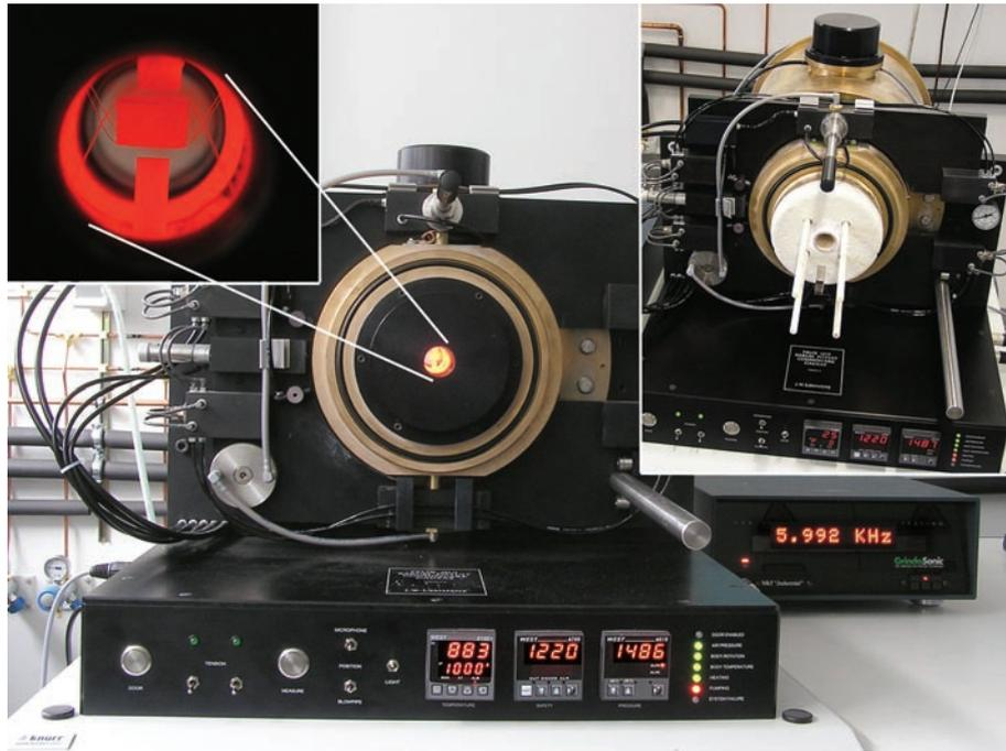
Fig. 16: „Grindo Sonic“ system for measurement of elastic moduli in the temperature range between 20 °C and 1200 °C.
