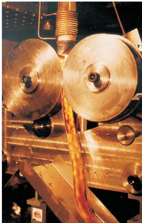
Fig. 1: Demonstration of temperature spottiness in a laboratory twin roll caster; strip width 6.5 cm.
