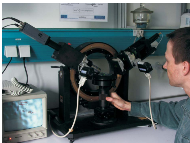
Application of a „Multiskop“ which combines one-wavelength, multi-angle ellipsometry, surface plasmon spectroscopy (SPS), waveguide modes, imaging ellipsometry, and SPS microscopy in a single modular set-up.
