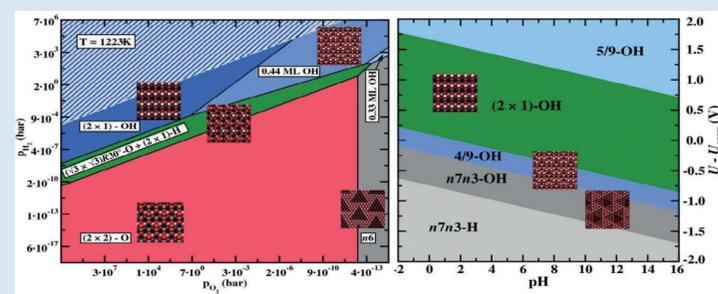
Surface phase diagram for a ZnO(0001)-Zn surface in equilibrium with a humid oxygen atmosphere at  $T=950^{\circ}\text{C}$  (left) and an electrochemical environment at  $T=300^{\circ}\text{C}$  (right). Geometries of the stable surface structures are shown as insets. Equilibrium conditions under which water would condensate on the surface are indicated by a white hashed area in the left picture.
