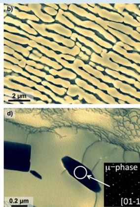
Evolution of the single crystal Ni-base superalloy during high temperature service: (a) SEM micrographs of the initial microstructure,  $\gamma'$  cubes in the  $\gamma$  matrix; (b) rafted microstructure after creep (160 MPa at  $1050^{\circ}\text{C}$ , 1% strain) and, (c) nucleated topologically close-packed (TCP) phases in the dendritic regions. (d) TEM micrograph showing a TCP particle and its corresponding electron diffraction pattern.
