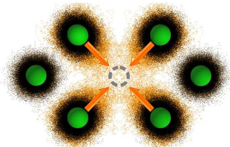
The picture shows the distribution of atoms next to a defect in a copper crystal at its melting point ( $1084^\circ\text{C}$ ). The green spots show the positions of the atoms at the absolute zero point. The dashed grey circle in the middle shows a lattice vacancy, a place where one atom is missing in the lattice. At
