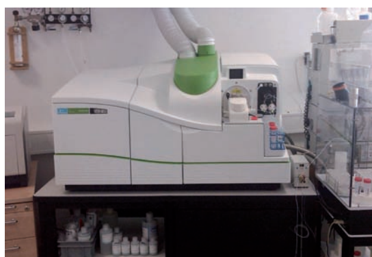
left: Nexion TM 300 ICP-MS; right: First un-optimized calibration measurement for Cr, Ni and Mn; integration time 1 s; matrix 0.1 mol l -1 NaCl; dispenser PFA 20 µl/s.
