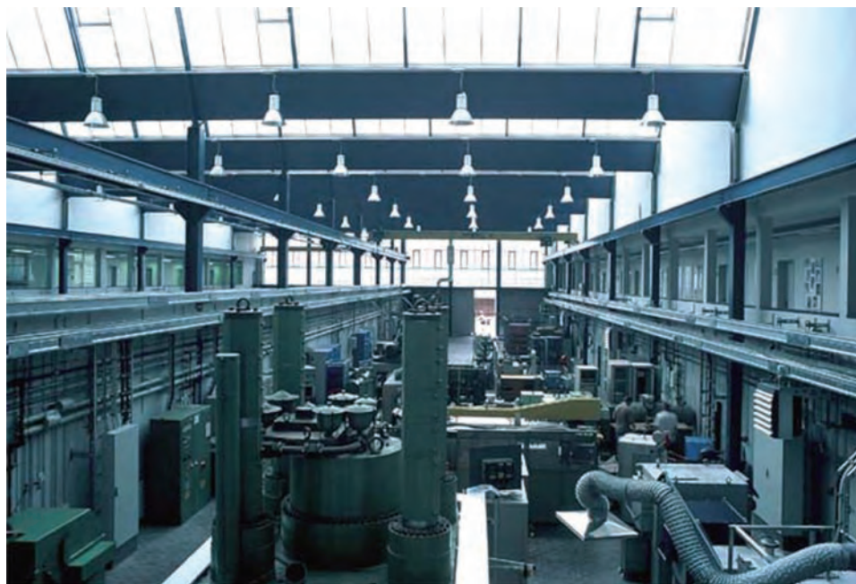
Renovated hall 8 showing facilities for thermomechanical treatment and metal forming; the large device in the foreground is the WUMSI (Warmumformsimulator, hot working simulator) (Photo: O. Schoplick, Düsseldorf).
