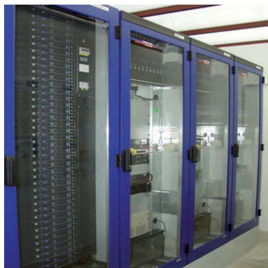
High-performance computer cluster with 320 CPU cores, 960 GB Ram, and 24 TB HDD integrated in water-cooled rack systems.
